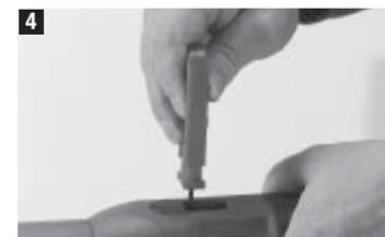
Clean the left and right-hand cartridge strip guideway twice, using the enclosed scraper.
