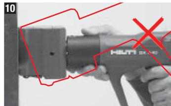
When marking, position the tool at right angles to the work surface, press forward on the tool and then pull the trigger.
