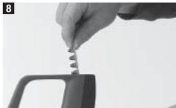
Load the cartridge strip narrow end first by inserting it into the bottom of the tool grip until flush. If the strip has been partly used, pull it through until a live cartridge is in the chamber.
