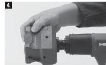
Firmly press the marking head onto the piston guide, then screw it on until it clicks into place.
