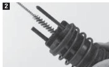
Clean the two holes in the cartridge chamber end-face using a small brush. Exhaust gas piston return system must be cleaned outside and sprayed sparingly with Hilti lubricant.
