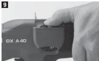
Adjust the driving power by turning the regulating wheel:
