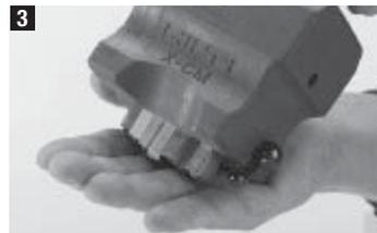
3 Remove the marking characters by turning the locking lever to the unlocked position.
