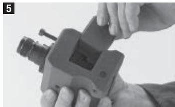
5 Remove the breech from the marking head.
