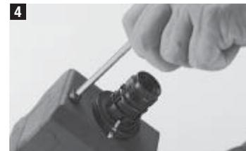
4 Unscrew the locking screw M6x30 approximately 15 times with an Allen key.
